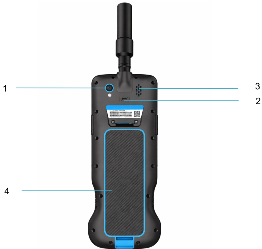
Figure 1-2-2 the backside of the A2
