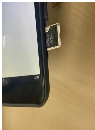
Figure 1-4-8 Installation of Micro SD card
